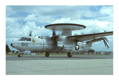
Sensors / EW: - AN/APS-125 - (1978) Radar, Radar, Air & Surface Search, 3D Long-Range, Max range: 463 km - AN/ALR-59 PDS - (1978) ESM, ELINT, Max range: 926 km
