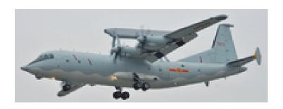
Sensors / EW: - KJ-200 Radar - Radar, Radar, Air & Surface Search, 3D Long-Range, Max range: 453.7 km
