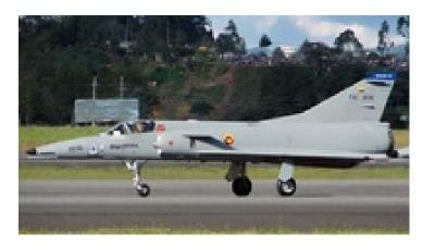
Sensors / EW: - EL/M-2001 RO - Radar, Radar, Range-Only (RO), Max range: 14.8 km - EL/L-8361 Elisra - ESM, RWR, Radar Warning Receiver, Max range: 222.2 km
