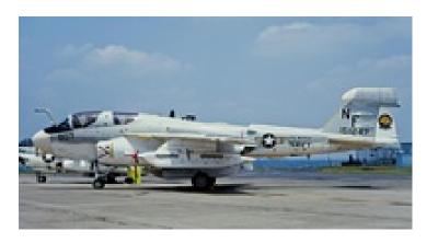
Sensors / EW: - AN/ALQ-126A - ECM, DECM, Defensive ECM, Max range: 0 km - AN/APS-130 - Radar, Radar, Surface Search, Medium-Range, Max range: 277.8 km
